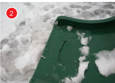
This tear could be an entanglement hazard.
