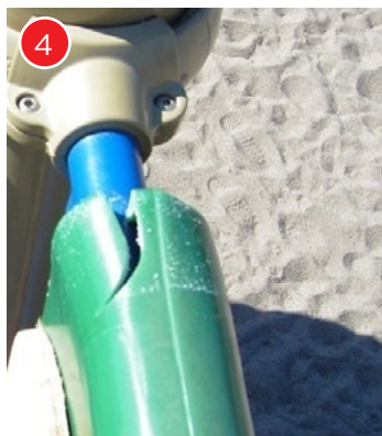
This cracked component is a hazard.
