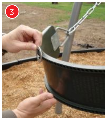
Test swings for protrusion hazards with this special gauge.
